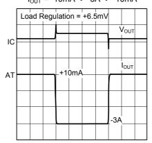
Ch1 :  $V_{OUT}$ , 20mV/Div, DC, Offset = 1.250V
