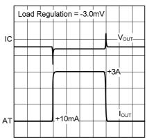
Ch1 : V<sub>OUT</sub>, 20mV/Div, DC, Offset = 1.250V
