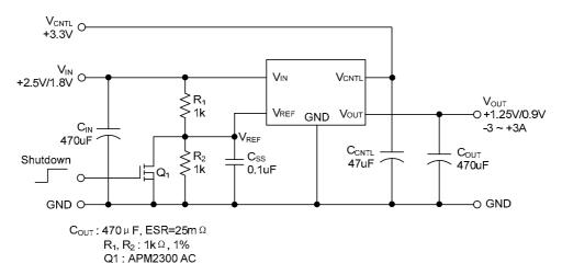
Note: Since R1 and R2 are very small, the voltage offset caused by the bias current of VREF can be ignore.
